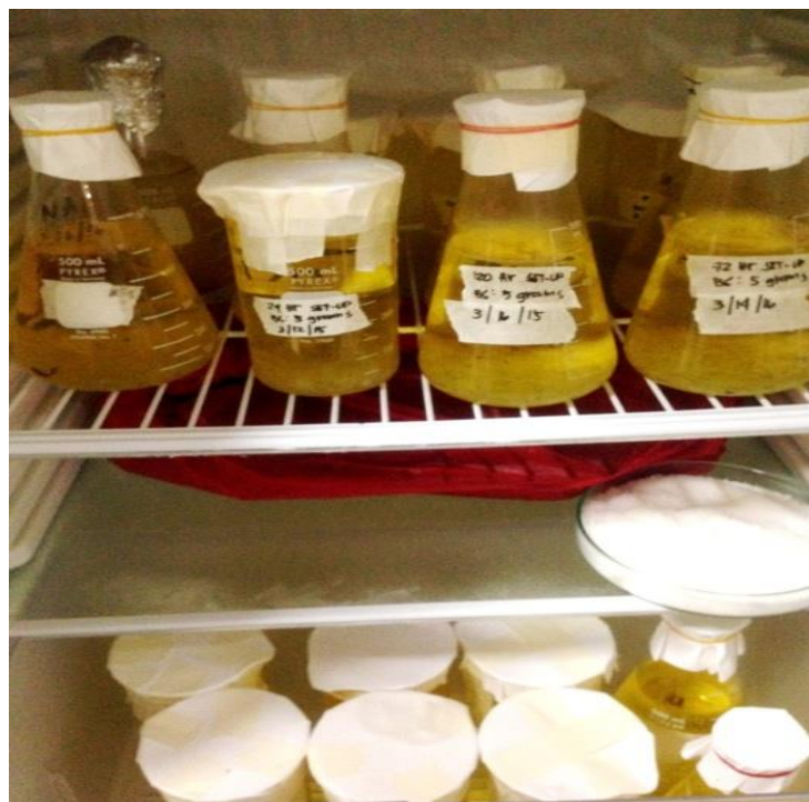
Figure 3: Samples with varying contact time and amount of biosorbent in triplicates
