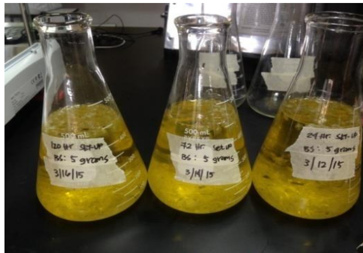
Figure 2: Exposure of biosorbent to synthetic wastewater with varying contact time
